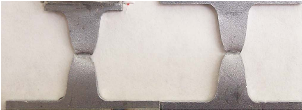
Fig. 4. Specimens after tensile tests at nominal strain rates of 750/s (left) and of 0.001/s (right).
