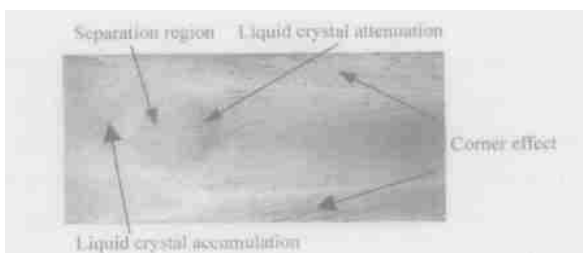
Fig. 5 Detailed photo of side wall separation region
