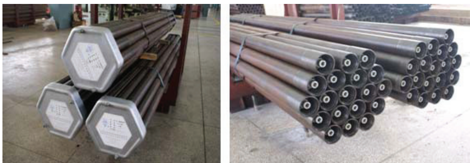
Fig.3. Drill rod with cable assembly inserts
