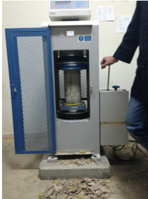
Fig. 7. Concrete Cylinder Testing Machine.
