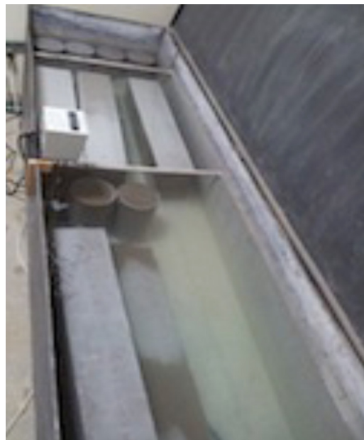
Fig. 6. Curing in the Water Storage Tank for 28 Days.
