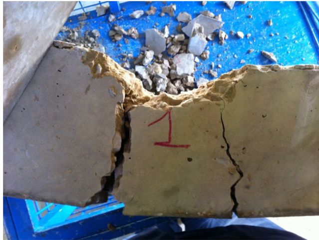
Fig. 9. Failure of a Monolithic Beam with a Construction Joint.
