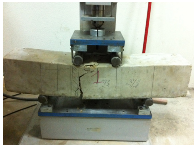
Fig. 8. Four Points Beam Testing Setup.
