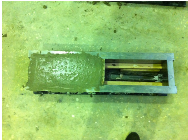
Fig. 3. Beam with a Construction Joint.
