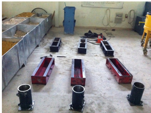
Fig. 1. Mold Form Preparation.
