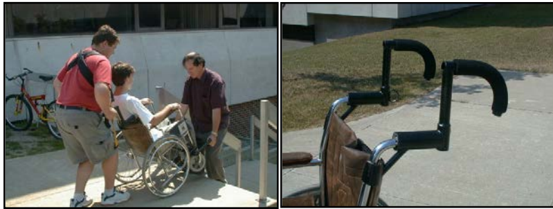
Fig. 3. (a) Prototype of an aid for transporting wheelchairs (b) Configuration of the upper handles
