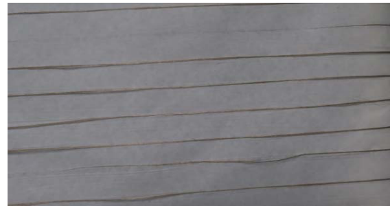
Fig. 6. Reinforcement sample produced with 10 roving, one inch spacing between each
