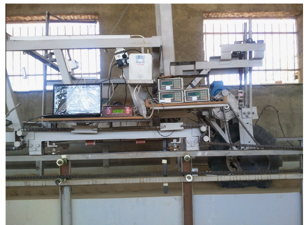
Figure 1 A general view of the single-wheel tester inside a capacious soil bin facility.
