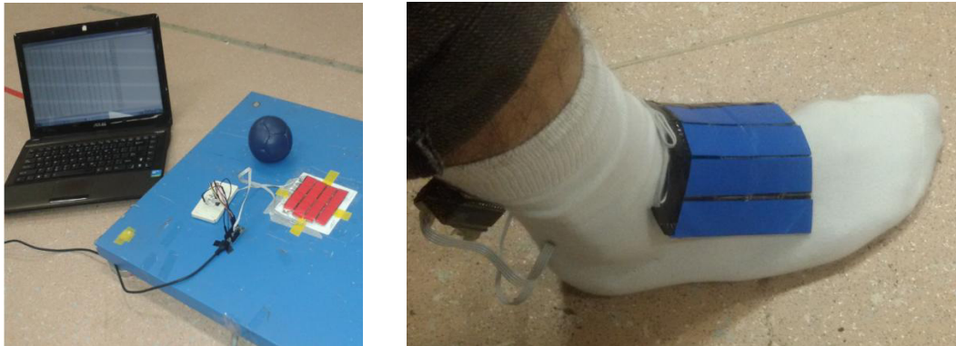
Fig. 1. Test set-up of the instrumented soccer footwear; left: a 4x4 multi-node system placed on Kistler force plate; right: system placed on the instep part of the foot for kicking tests
