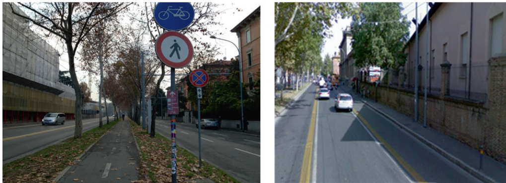
Figure 3. The off-street facility and roadway layout in Segment 1 “Ercolani” (N.B.: the red circled sign with the pedestrian indicates pedestrians are technically prohibited from the facility).
