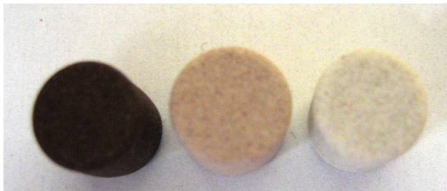
Fig. 4. Smelting samples of Q3 before treatment, followed by magnetic separation and bioleaching with washing process.
