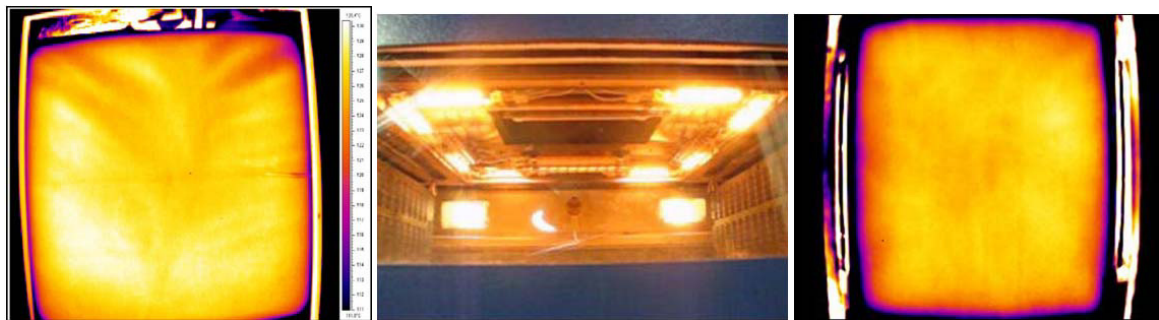
Fig. 7. (left) IR camera image of part bed with two-zone heating elements; (center) photograph of multi-zone heater layout; and (right) IR camera image of part bed with multi-zone heaters. Images courtesy of Tim Gornet, Additive Manufacturing User’s Group (Tucson, AZ, USA).
