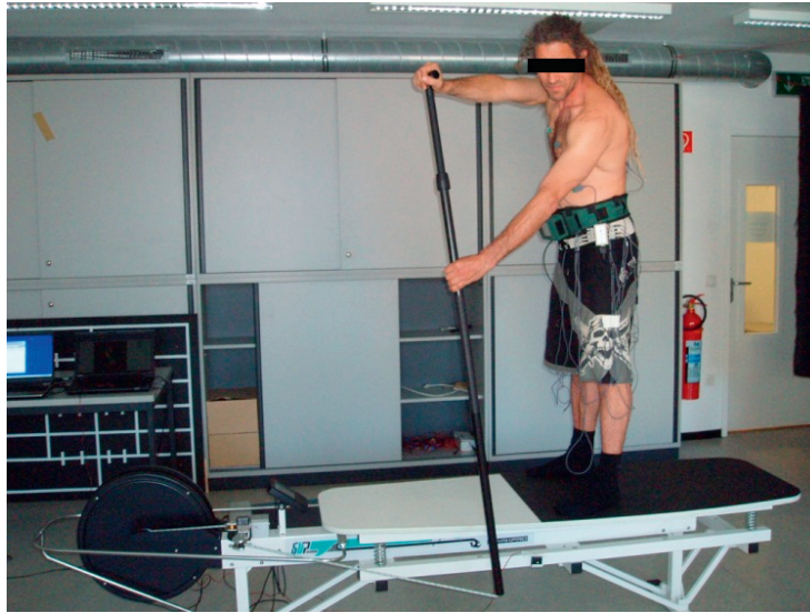
Fig. 1. SUP ergometer during laboratory tests, subject is equipped with 16 bipolar sEMG electrodes and currently in the power phase
