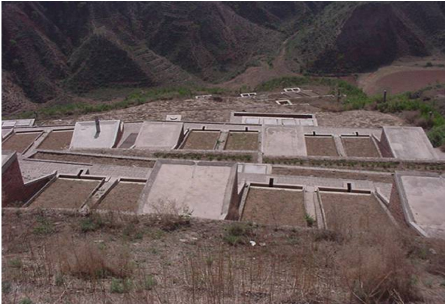
Fig. 3. Short slope plots (SSP) with a dimension of 2 m wide and 7 m long at slope angles of 5°, 10°, 15°, 20°, 25°, and 30°.
