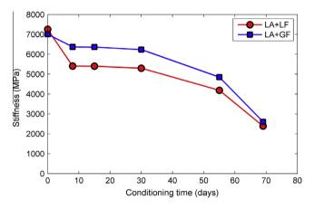
**Fig. 3.** Sample predicted stiffness degradation of asphalt mixtures using exponential sigmoidal model in Eq. (2). Data were from mixtures containing 4% nominal air voids. The shapes of the plots are typical of cohesively dominated stiffness degradation resulting from a plasticization process.
