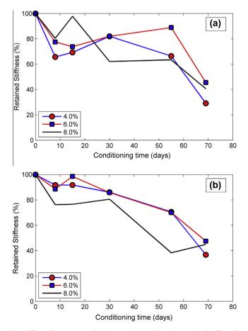
**Fig. 2.** Effects of moisture conditioning and air void levels on retained stiffness for asphalt mixture tested at 20 °C. The unique sigmoidal shape of the stiffness degradation curves could be used to characterize mixture sensitivity to moisture. (a) LA + LF. (b) LA + GF.
