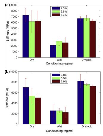
**Fig. 4.** Stiffness of asphalt mixtures (LA + LF and LF + GF) subjected to three conditioning regimes showing reversible moisture-induced stiffness degradation. Dry = original specimens without moisture exposure; Wet = specimens subjected 69 days of moisture conditioning at 60 °C. Stiffness was determined at 20 °C. Each mixture type (LA + LF or LF + GF) was compacted to three different nominal air voids 4%, 6%, and 8%. (a) LA + LF. (b) LA + GF.
