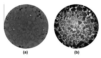
**Fig. 7.** Micro CT scans of dense graded asphalt mixture. (a) Original image, brighter areas represents aggregates. (b) Segmented image showing mastic moisture diffusion paths (white areas) around the aggregate (darker areas) particles. Diameter of specimen approximately 100 mm diameter.
