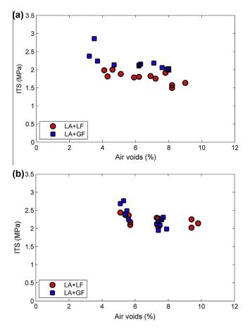
**Fig. 5.** (a) Indirect tensile strength of asphalt mixtures conditioned in water at 60 °C for 69 day and then dried for 47 days (=116 days of conditioning). (b) Indirect tensile strength of asphalt mixtures conditioned in at ambient conditions (20 °C and 50% RH) for 116 days. Tensile strength was obtained using a loading rate of 20 mm/ min and a testing temperature of 20 °C.
