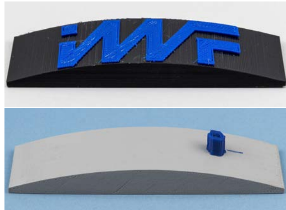
Figure 5. Base workpiece examples printed by a commercial 3D-printer (black/grey) with blue structures added by CAD/CAM-driven partial additive manufacturing using HEXA II.
