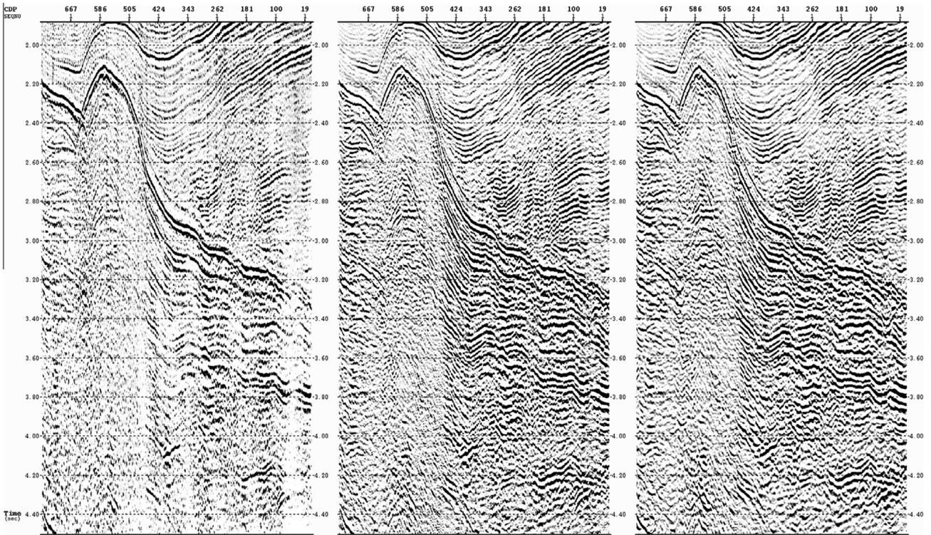
**Fig. 3.** Original scanned seismic section converted to SEG-Y (left). Same data processed to correct amplitude anomalies from the scanning process and restore continuity of the signal using the Tau-P transform (center). Final migrated section (right).
