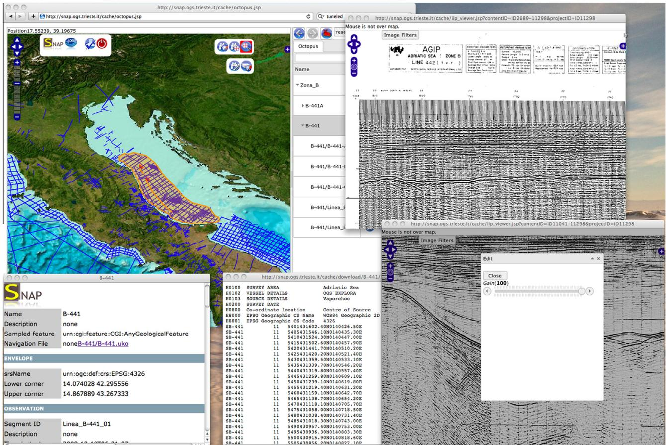
**Fig. 8.** SNAP, the OGS web based data access system. Seismic data can be searched geographically and textually (upper left). Once data are found it is possible to read their metadata (lower left) and download positioning in a UKOOA file (lower center). Data can be visualized either as a static image file (upper right) or as actual Seg-Y data, where basic processing on the data is possible (lower right).
