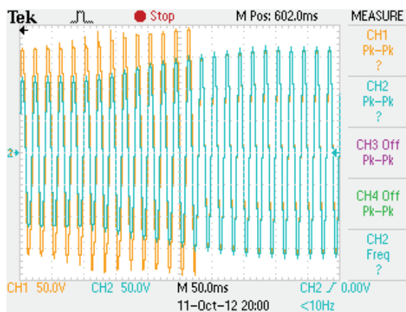
Fig. 21. Input and load voltage duration before the end of voltage sag.
