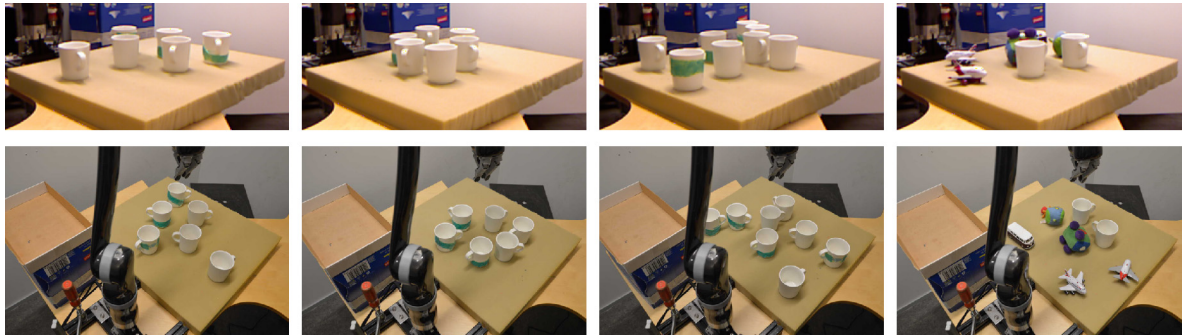
Fig. 9. Top row: cropped kinect images of the four scenes used in the robot arm experiments. Bottom row: corresponding photographs of the scenes. Each scene contains “dirty” (partly green color) and “clean” objects. Scenes one to three contain only cups but scene four contains also several toys. (For interpretation of the references to color in this figure legend, the reader is referred to the web version of this article.)
