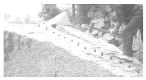
Fig. 5 Series of small holes along the line of fracture plane with inserted steel chisel
