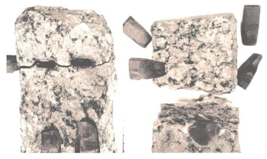
Fig. 10 Fracture surface passing through the proposed fracture plane
