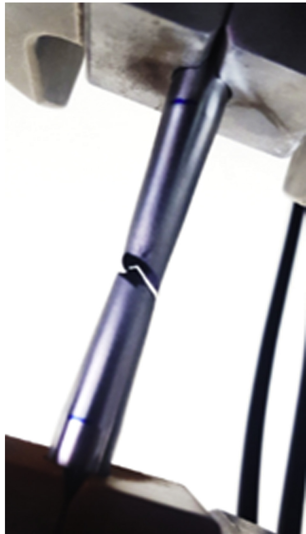
Fig. 2 – A PM Mo tube sample tested at room temperature. PM, power metallurgy.
