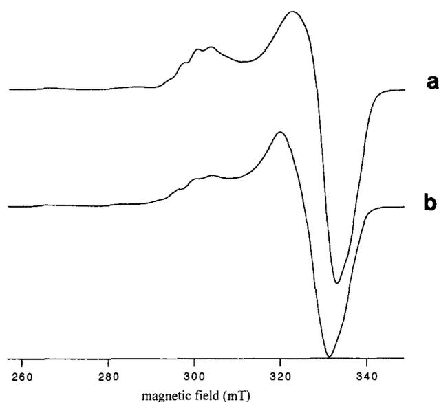
Fig. 2. X-band EPR spectrum at 23 K and using a power level at which the type II signal is saturated (20 mW) of (a) the  $\text{Cu}_A$ -containing amicyanin mutant in 25 mM HEPES (~40% glycerol) at pH 7.0 and (b) the  $\text{Cu}_A$  domain of cytochrome *c* oxidase from *B. subtilis* in 20 mM Tris buffer (10% glycerol) at pH 8.0.
