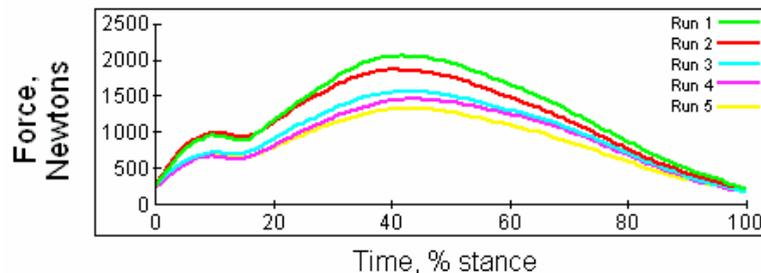
Fig. 1. With each run during the 5 x 1.5 minute test the output of the pressure insole decreased gradually
