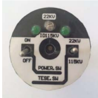
Fig. 9. The front of the induced voltage detector
