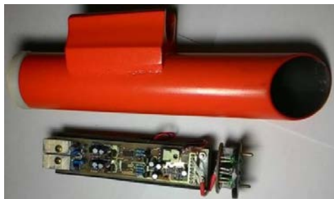
Fig. 11. Induced voltage detector.
