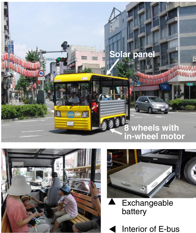
Fig. 10. Photographs of low-speed E-bus during a road test.
