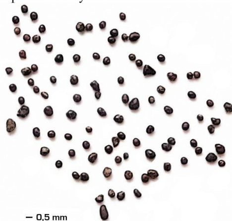
Fig. 2. Photo of iron concentrate particles.
