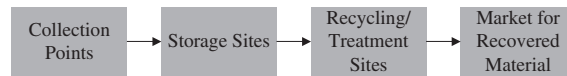
Fig. 1 Material Flow from site to site in the formal waste sector if e-waste (based on the work of Shih [16])
