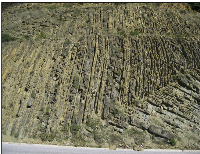
Fig. 1. Moderately disturbed rock mass with sandstone and siltstone alternations in similar amounts.
