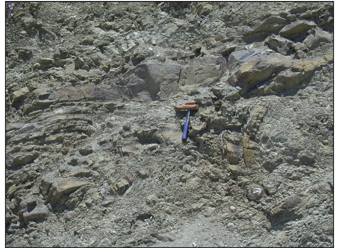
Fig. 2. Tectonically disturbed sheared siltstone with broken deformed sandstone layers. These layers have almost lost their initial structure, almost a chaotic structure.
