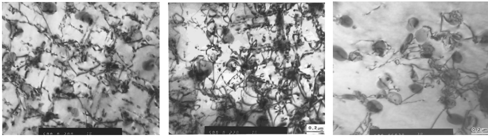
(a) T6 + 250°C x 0-hour aging, Nf=530 (b) T6 + 250°C x 10-hour aging, Nf=870 (c) T6+aging time 100hrs, Nf=1700
