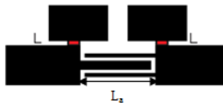
Fig. 1. UWB Filter with chip inductors 5
