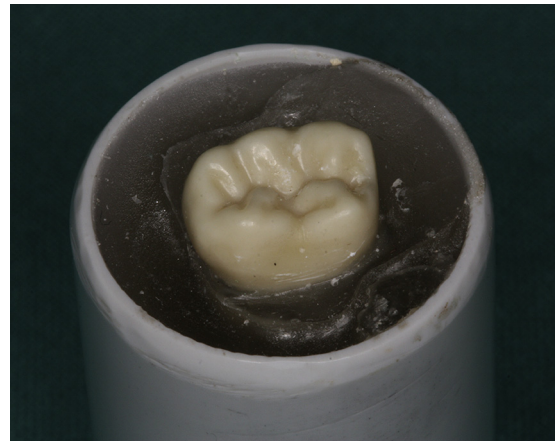
Fig. 3 – Simulated occlusal table of 120° without PDL-simulator (rigid model).
