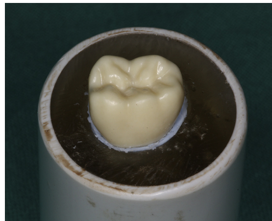
Fig. 4 – Simulated occlusal table of 120° with PDL-simulator (resilient model).
