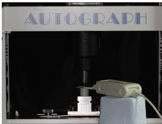
Fig. 6 – Table of 180° mounted on the Autograph®, AG-I with the T-Scan®III HD sensor interposed and being loaded.
