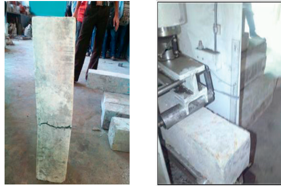
Fig 5 Testing of specimen under Flexure
