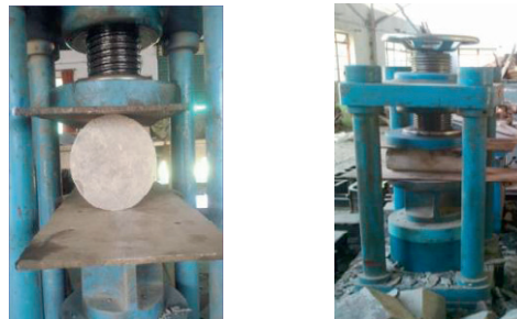
Fig 4 Testing of specimen under split tension
