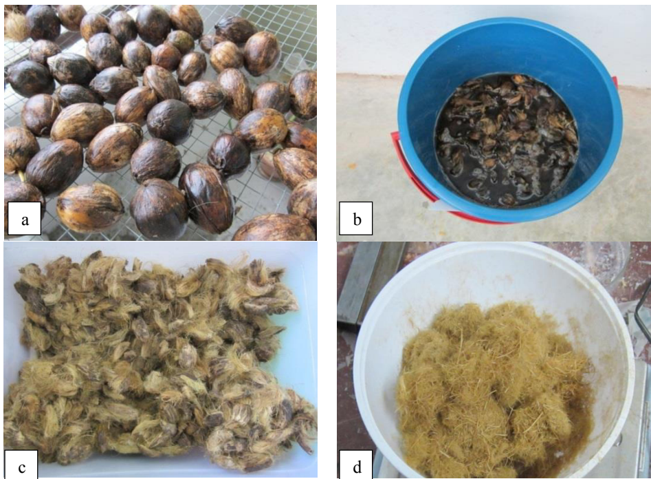
Fig.1. Step of betel nut fiber preparation a) Raw betelnuts, b) Betelnuts soaked in water for ripening, c) Extracted fiber, d) Random size fibers
