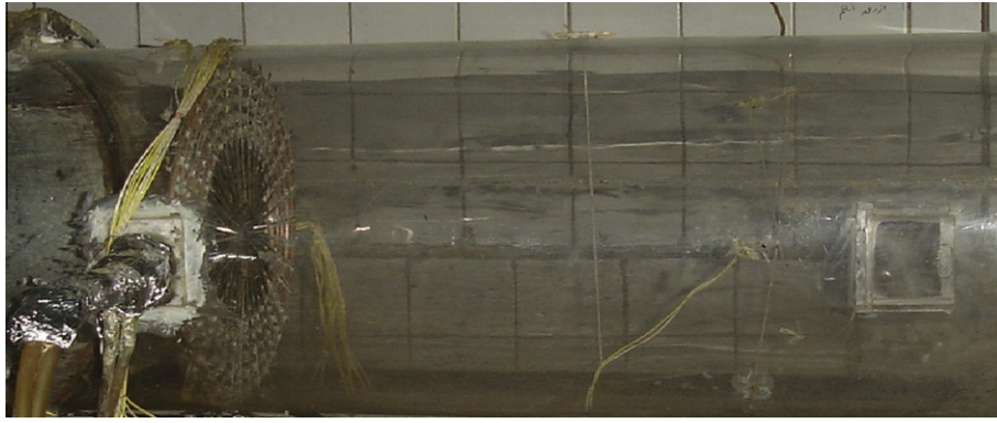
Figure 2 Photograph of the spiral coil inside the test section.
