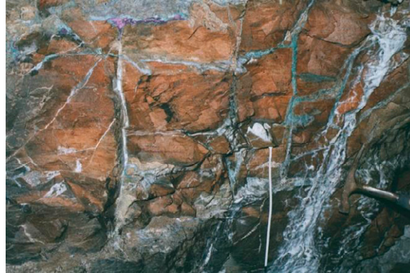
Figure 5: typical clogging of hyperalkaline groundwater flowpaths in the Bituminous Marl Formation of northern Jordan [26]. Note geological hammer, bottom right, for scale.
