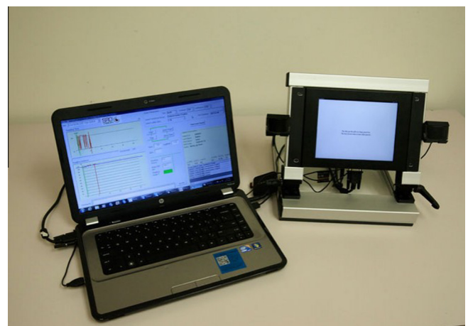
Fig. 9. The Salzburg Reading Desk uses modern computer technology to present text in random order while measuring reading distance with IR cameras and reading speed with voice detection.
