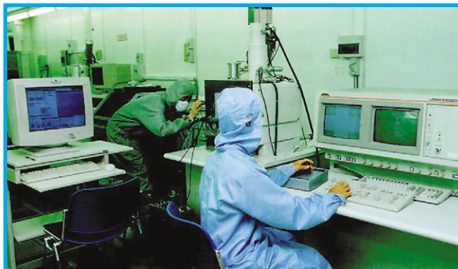
Deep Submicron high-frequency transistor fabrication using Raith + Jeol direct electron beam writing
