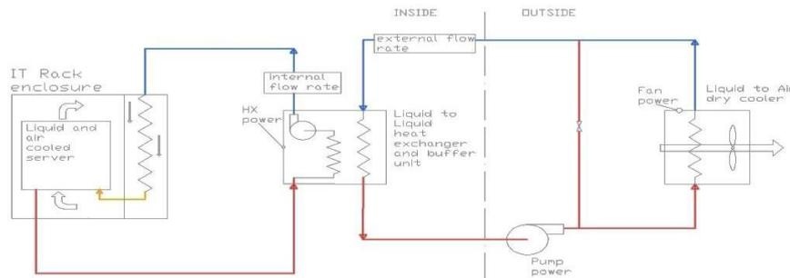
Fig. 1. Schematic of the liquid cooling design.
