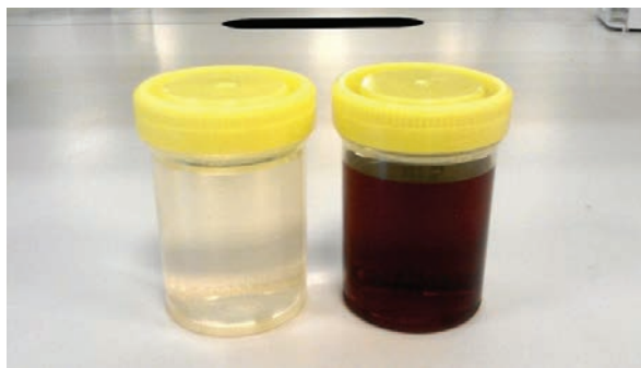
Fig. 9. Picture of the aqueous 30 wt.% MEA after 3 weeks at 40 °C and sparged with CO 2 and air. The sample in the left container was not exposed to UV light. The sample in the right container was exposed to UV light
