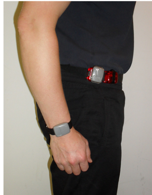
Fig. 1. Accelerometer locations at the waist and right wrist: GT1M and GT3X+ accelerometers adjacent and the GENE taped to the GT1M, positioned over the right hip; GENE on right wrist.
