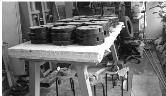
Fig. 3. Loading of CLT plate by the load with intensity equal to 7.5 kN/m 2 .
