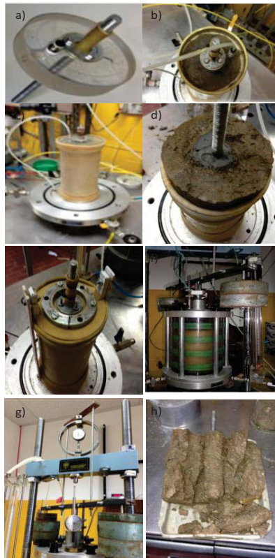
Fig. 3. Pull-out test apparatus: a) plexiglass plate for injection; b) top plan view of the plate connected to the cell; c) front view of the plate; d) setting of the cement in the cell; e) plate for the pull-out test and steel bars; f) loading system; g) loading ring and micrometer; h) injection bulb.
