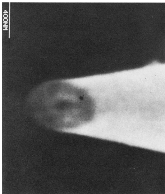
FIGURE 4 A scanning electron micrograph of the tip of a metallized pipette is shown with a 5,000 \text{ \AA} outer diameter and with a <1,000 \text{ \AA} central aperture. Although even smaller apertures could be prepared with our technique, they would be difficult to characterize with the limited resolution of the SEM available.
