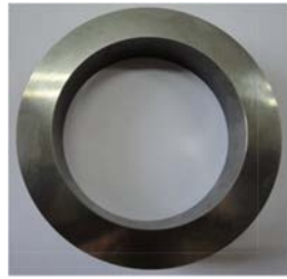
Fig. 1. Photo of IBSP processed WC-Ni cemented carbide mechanical seal where the outer diameter is 150 mm.
