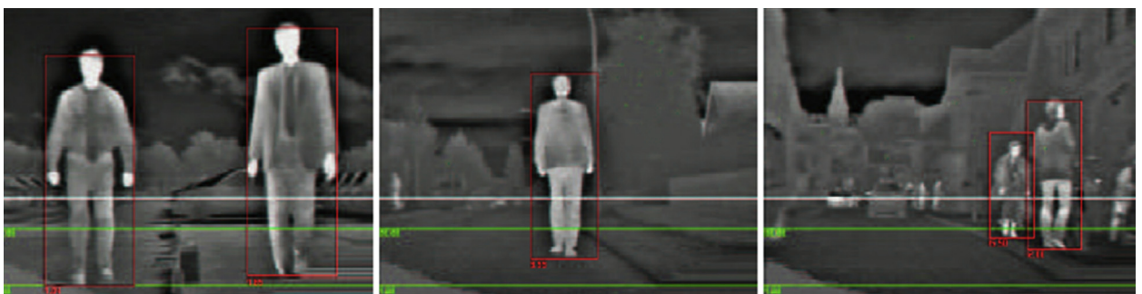
Fig. 3. Sample results of pedestrians' detection ( Bertozzi et al., 2003 ).
