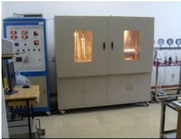
Fig. 1 The test system of gas and liquid relative permeability in coal
