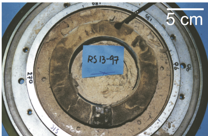
Fig. 15. Top view of a clay smear formed in ringshear experiment (Sperrevik et al., 2000) after brushing away top sand layer. Dark block at bottom of photo (inner ring) is source clay layer.
