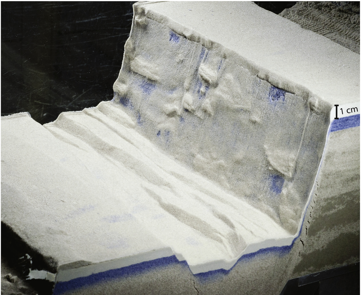
Fig. 21. Excavated surface of sheared clay layer showing different degrees of mixing of clay with sand from both sides of the clay (light blue areas of fault) and holes in clay gouge (center of dark blue areas). Technique described by Noorsalehi-Garakani et al. (2013). Note sheared lenses in the master shear zone (thicker, pure white sections on fault surface).
