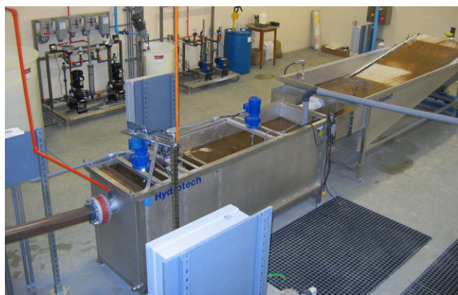
Fig. 1. An inclined belt filter (IBF) and coagulation–flocculation tank operated for microscreen drum filter backwash dewatering at the Craig Brook National Fish Hatchery (East Orland, ME). Photo background shows alum and polymer dosing systems and chemical reservoirs (in background).
