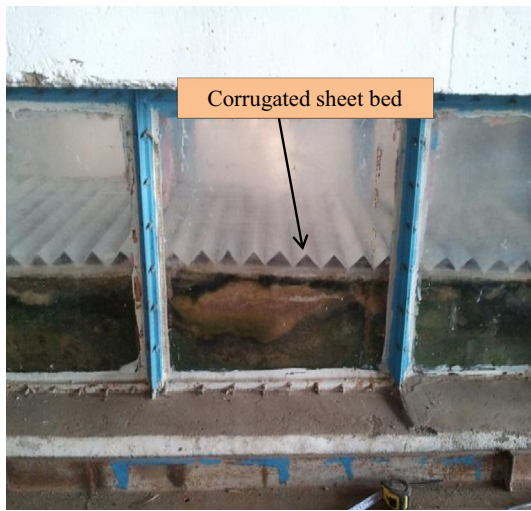
Figure 3 Plexiglas's wall section.
