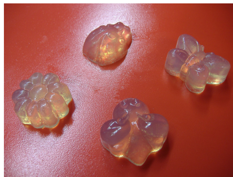
Fig. 6. Shaped transparent 10% (40% \beta -sitosterol + 60% \gamma -oryzanol) oleogels in sunflower oil. No special processing was required: dissolved \beta -sitosterol and \gamma -oryzanol in sunflower oil was poured in a standard silicone chocolate mold that was cooled in a fridge.
