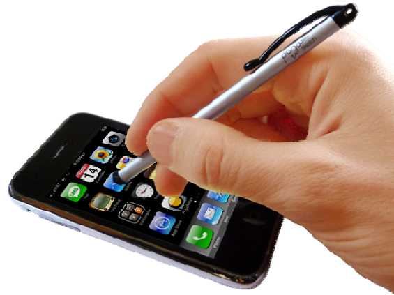
Figure 3. Example of using a touch pen for capacitive screen: It also covers the screen partially [3].
